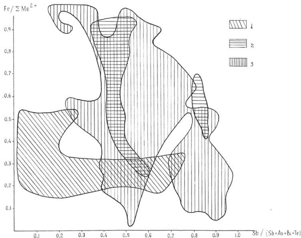
Fig. 1. The variation of the \text{Fe}/\Sigma\text{Me}^{2+} ratio and \text{Sb}/\Sigma\text{Sb} + \text{As} + \text{Bi} + \text{Te} ratio in fahl-ore in the gold deposits from Middle Asia.
